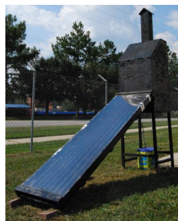
Plate 2: Solar Convection Dryer (Schivavone et al. , 2013)
