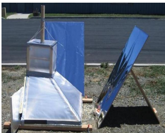
Plate 1: Solar Dryer with Two Solar Concentrating Panels (Stiling et al. , 2012)
