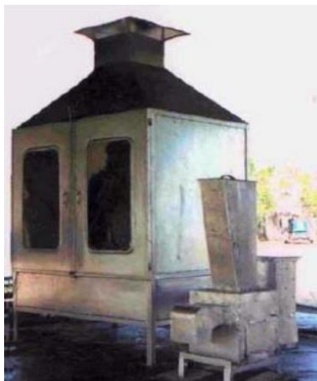
Plate 3: Solar-Biomass Hybrid Cabinet Dryer (IAE/UPLB, 2002)
