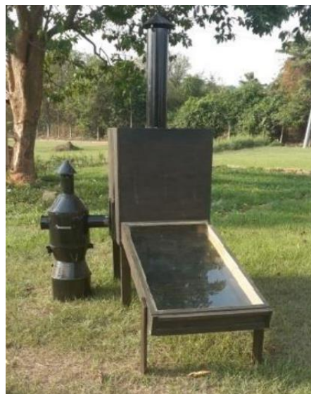
Plate 4: Solar-Biomass Convective Dryer (Tibebu, 2015)
