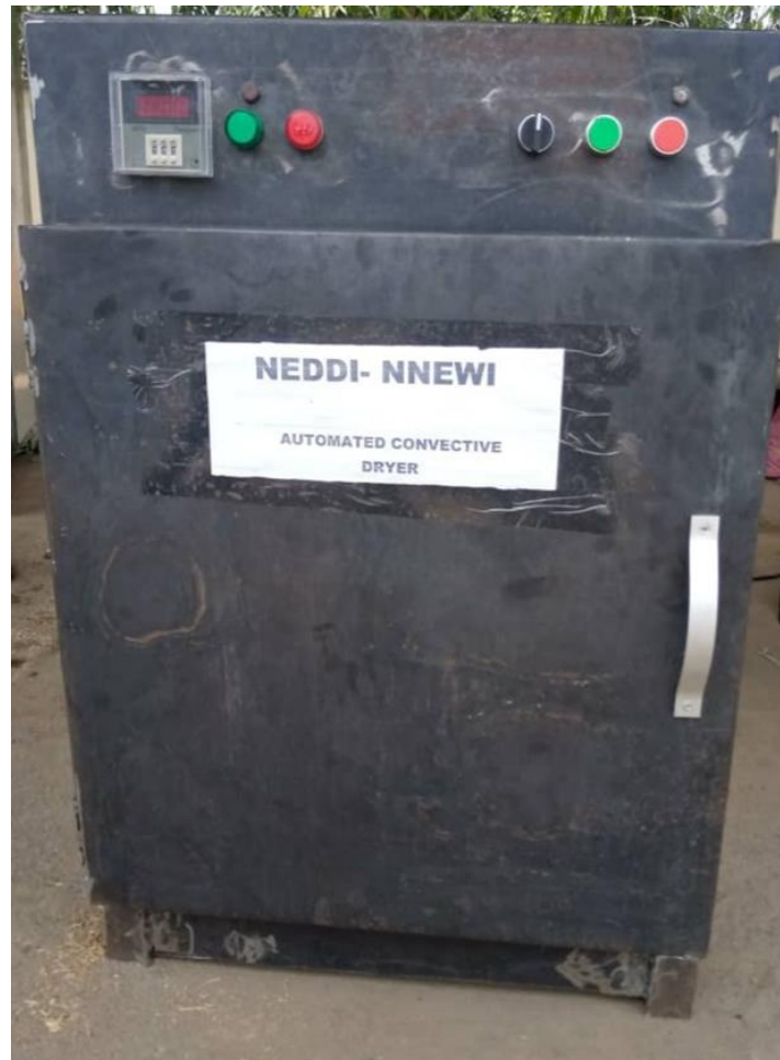
Plate 5: Regulated Convective Compartmental Dryer.
